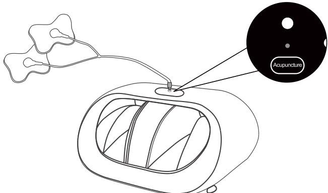
The interface cable into the jack corresponding to the operation panel.
