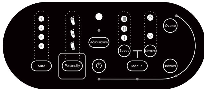
4、Manual The manual setting key can control "speed" and "direction". The product has 3 speeds which are low, middle and fast. The indicator light of each speed key has different colors. The direction key has two levels that are clockwise and counter clockwise revolution.
